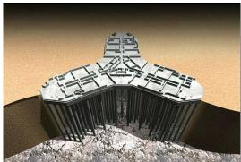
design of piled rafts supporting high rise buildings (generally based on expensive 3D finite element or finite different analyses) but also for that of ordinary buildings and bridges.
