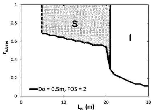
Figure 4. Design chart for a solid circular RC pile in loose sand ( $D_r = 35\%$ ):  $D_0 = 0.5\text{m}$ ,  $\text{FOS} = 2$ . From Madabhushi et al. (2009). In the blank areas the pile is verified, in those identified by “S” the pile encounter a crisis by bearing capacity while in those identified by “I” the crisis is because of instability.
