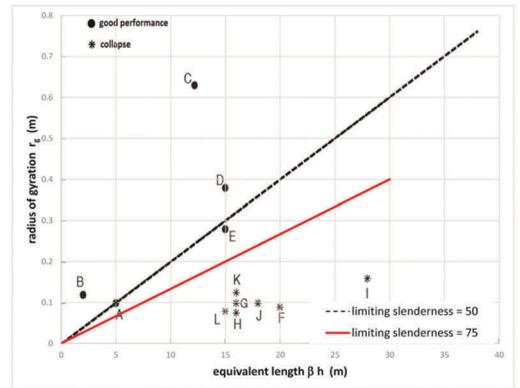
Figure 3. Admissible domain: measured performances of deep foundations after real earthquakes. From Bhattacharya & Lombardi (2012).
