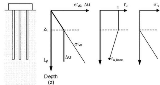
Figure 2. Effective stress conditions around piles for full liquefaction until  $z_L$  depth. From Madabhushi et al. (2009).
