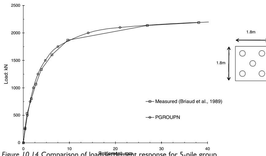
Figure 10.14 Comparison of load-settlement response for 5-pile group.
