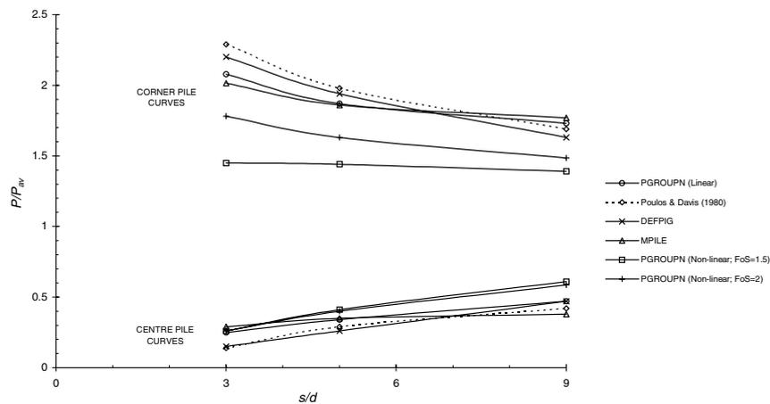
Figure 10.6 Comparison of axial load distribution to individual piles in  $5 \times 5$  pile group.
