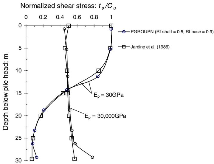
Figure 10.4 Comparison of shaft shear stress distribution for single pile at a load level  $P/P_u = 0.5$ .
