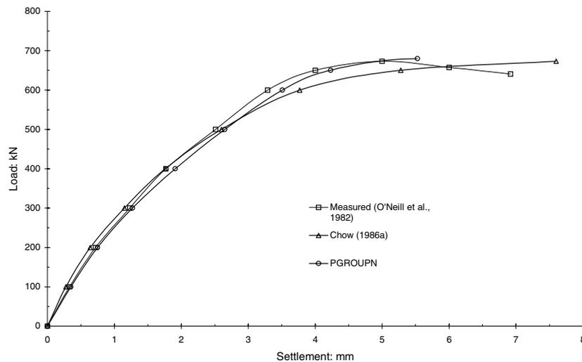
Figure 10.9 Comparison of load-settlement response for single pile.
