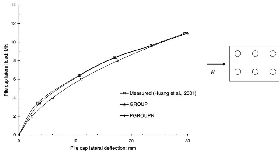
Figure 10.16 Comparison of load-deflection response for 6-pile group.
