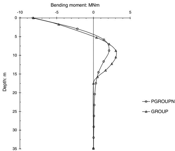
Figure 10.18 Comparison of moment profiles of leading row of piles in 6-pile group under the maximum applied lateral load  $H = 10,948$  kN.
