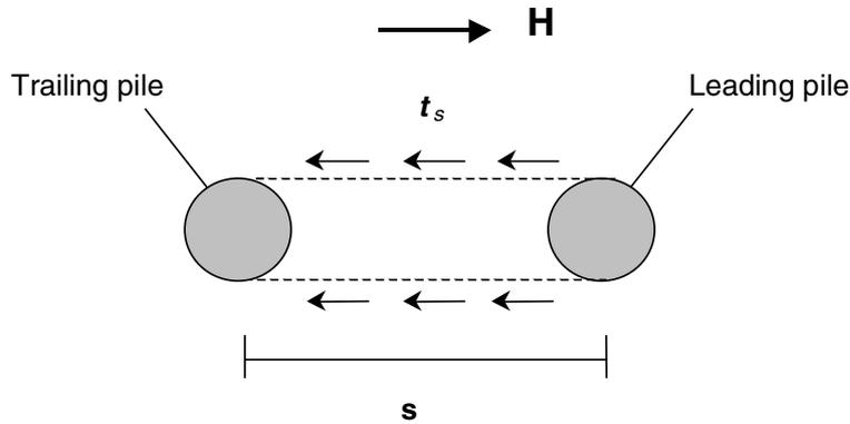
Figure 10.1 Plan view of block failure under lateral load (after Fleming et al., 1992).
