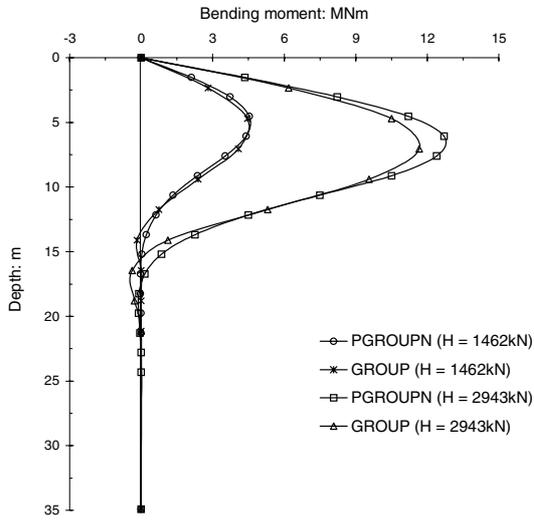
Figure 10.17 Comparison of moment profiles of single pile.
