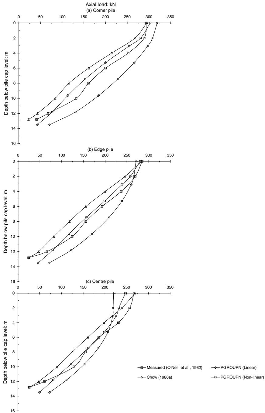
Figure 10.11 Comparison of axial load distribution in 9-pile group at a working group load of 2.58 MN (Note: Curves by Chow (1986a) were reported in Chow (1986b)).
