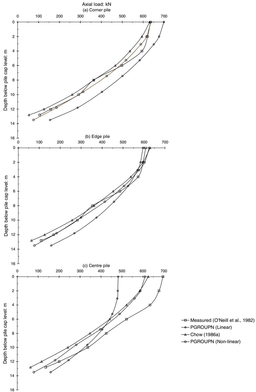
Figure 10.12 Comparison of axial load distribution in 9-pile group at a group load nearing failure of 5.66 MN (Note: Curves by Chow (1986a) were reported in Chow (1986b)).
