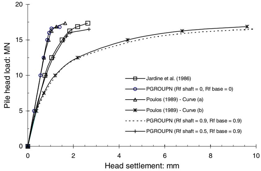
Figure 10.3 Comparison of load-settlement response for single pile ( $E_p = 30,000 \text{ GPa}$ ).
