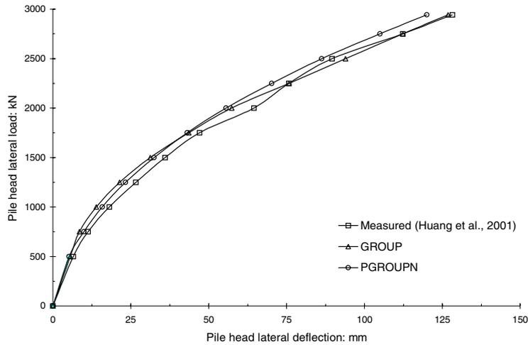
Figure 10.15 Comparison of load-deflection response for single pile.
