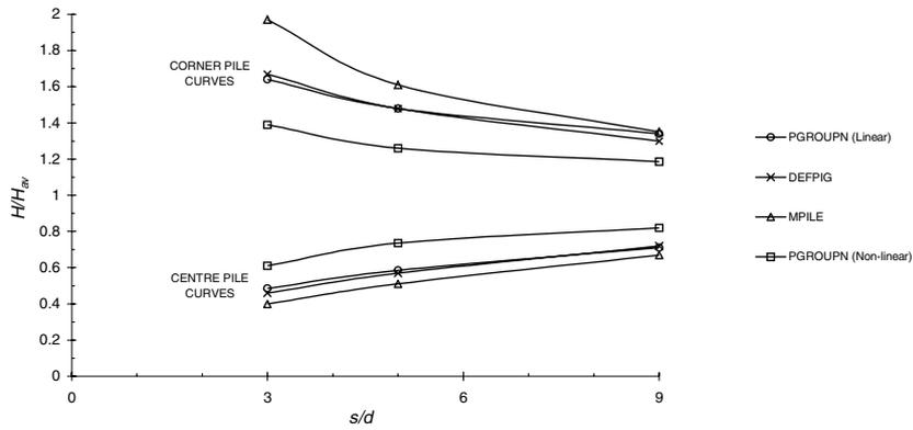
Figure 10.7 Comparison of lateral load distribution to individual piles in 5 × 5 pile group.
