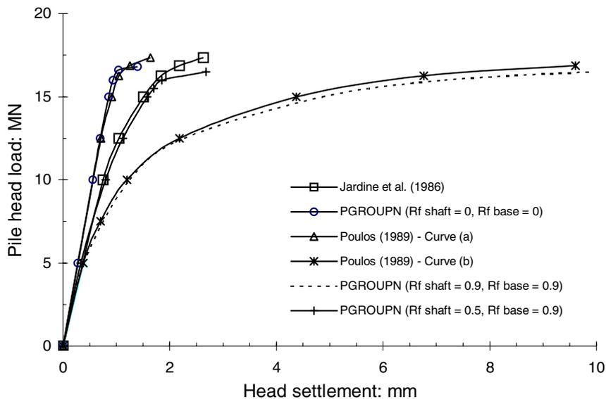
Figure 10.2 Comparison of load–settlement response for single pile ( $E_p = 30$  GPa).
