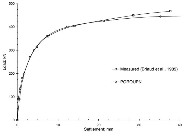
Figure 10.13 Comparison of load-settlement response for single pile.
