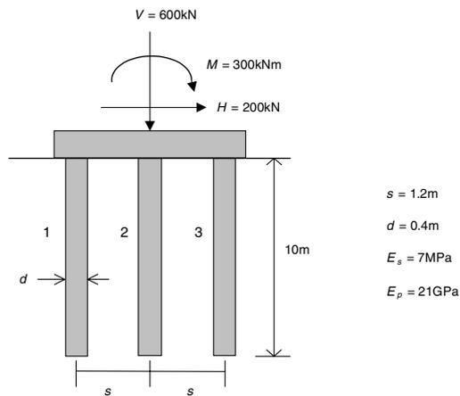
Figure 10.8 Group of 3 piles considered in comparison of methods.
