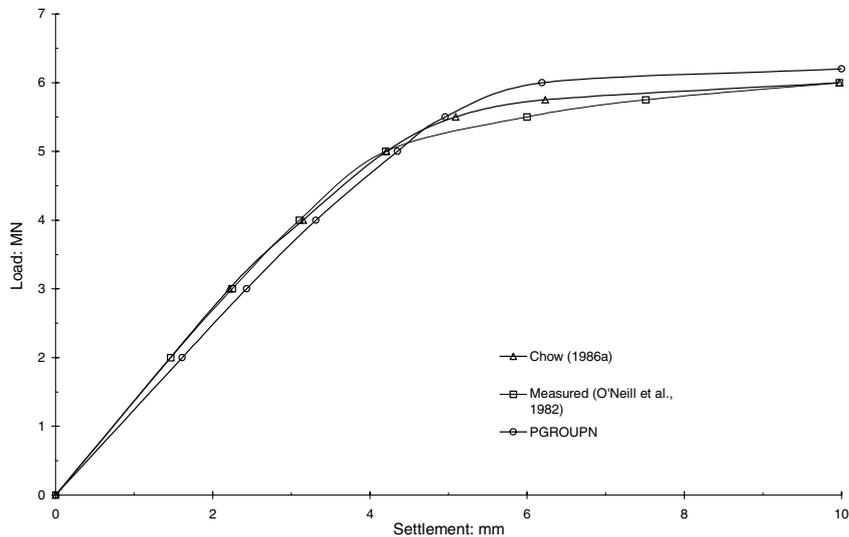
Figure 10.10 Comparison of load-settlement response for 9-pile group.
