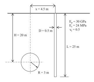
Fig. 2. Single-pile problem analysed.
