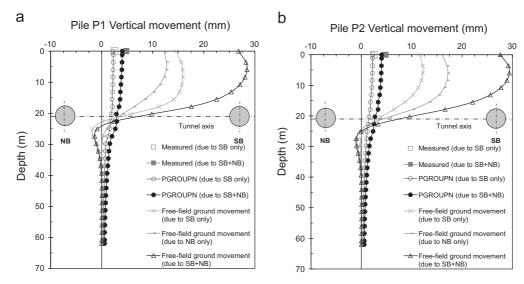
Fig. 17. Vertical movement profiles for (a) pile P1 and (b) pile P2.
