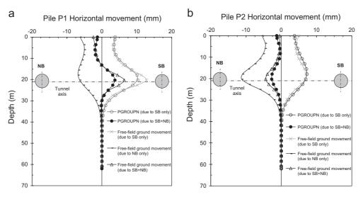
Fig. 18. Horizontal movement profiles for (a) pile P1 and (b) pile P2.
