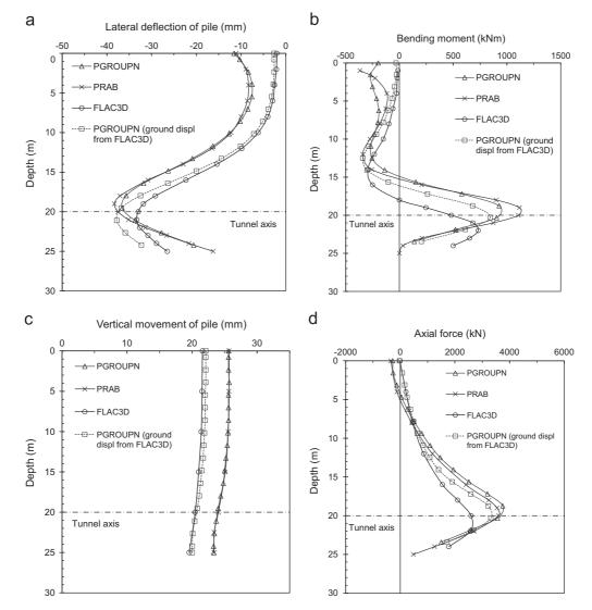
Fig. 8. Comparison of pile-group responses for front pile.
