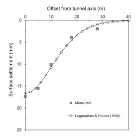
Fig. 12. Measured and computed free-field surface settlements.
