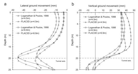
Fig. 7. Comparison of computed free-field ground movements.
