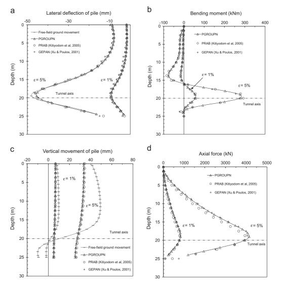
Fig. 3. Comparison of single-pile responses.
