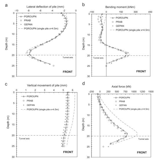
Fig. 5. Comparison of pile-group responses for front pile.
