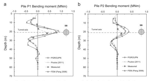
Fig. 16. Measured and computed bending moment distributions for (a) pile P1 and (b) pile P2.
