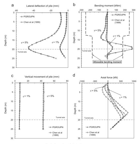
Fig. 9. Comparison of single-pile responses.
