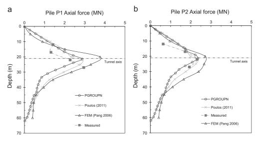
Fig. 15. Measured and computed axial force distributions for (a) pile P1 and (b) pile P2.
