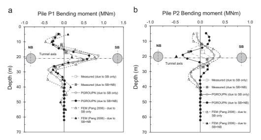
Fig. 20. Measured and computed bending moment distributions for (a) pile P1 and (b) pile P2.
