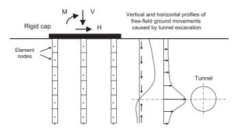
Fig. 1. BEM schematisation of the problem.
