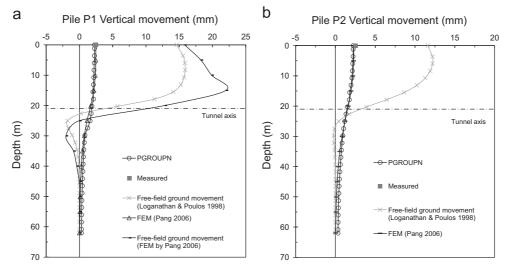
Fig. 13. Vertical movement profiles for (a) pile P1 and (b) pile P2.
