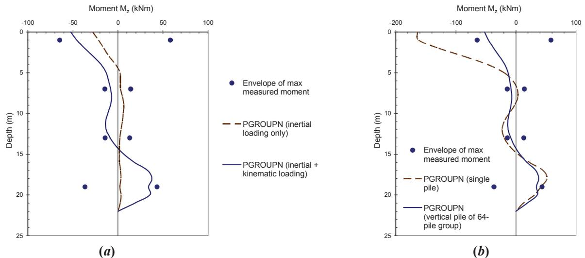
Figure 9. (a) Effect of kinematic and inertial loading; (b) Effect of group interaction
