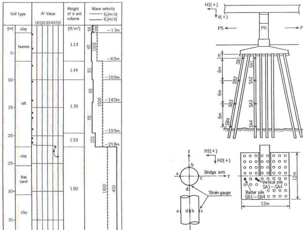
Figure 6. Ohba-Ohashi Bridge soil conditions and pile foundation (after Tazoh et al., 1987)
