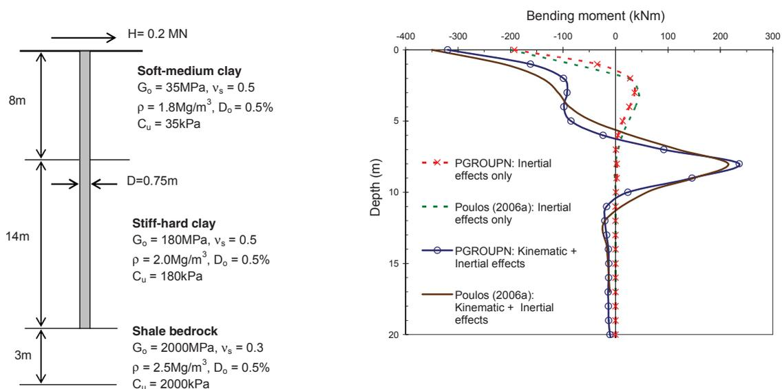
Figure 2. Comparison of bending moment with Poulos (2006a)
