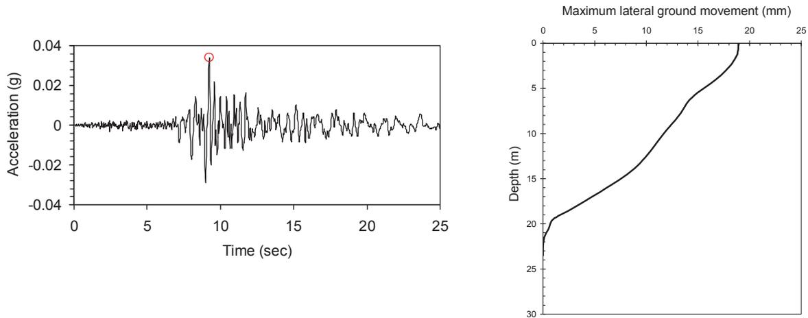
Figure 7. Recorded seismic motion at GB1 (H1 direction) and resulting maximum lateral ground movement profile from EERA
