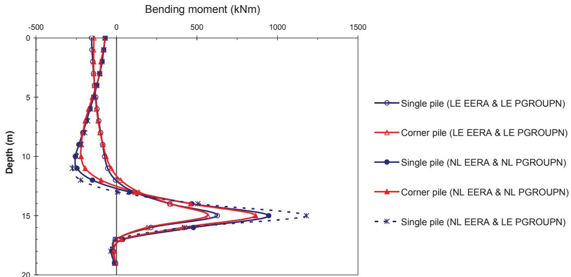
Figure 5. Influence of soil nonlinearity on kinematic bending moment
