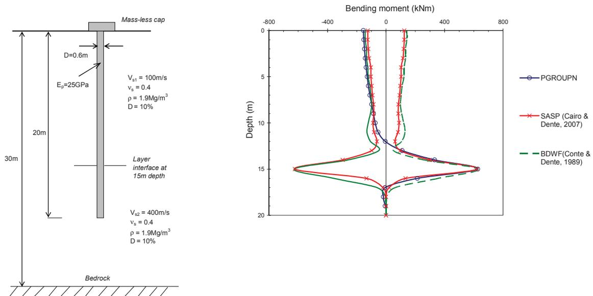
Figure 3. Comparison of kinematic bending moment with dynamic analyses
