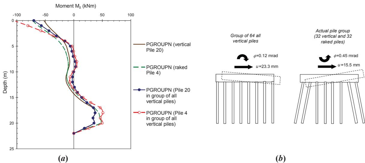
Figure 10. Effect of raked piles on (a) bending moment and (b) cap deflection and rotation
