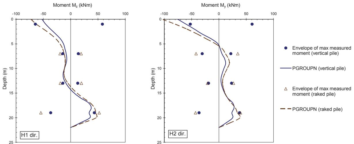
Figure 8. Comparison of bending moment in H1 and H2 directions
