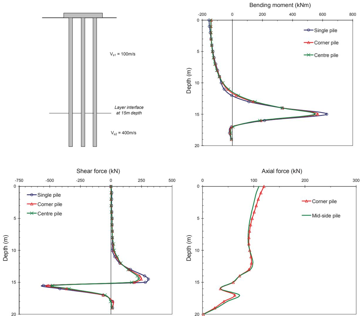
Figure 4. PGROUPN prediction of kinematic internal forces in 3x3 pile group
