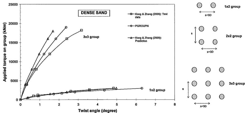
Fig. 16. Torque-twist angle curves for pile groups in dense sand
