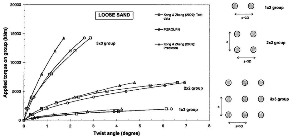
Fig. 15. Torque-twist angle curves for pile groups in loose sand
