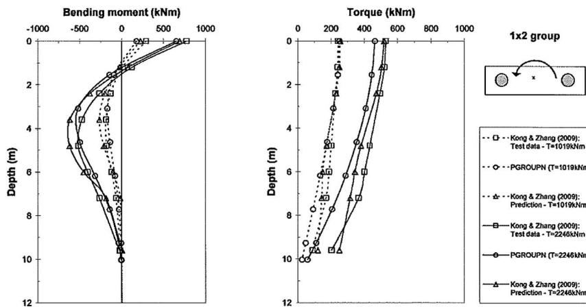
Fig. 18. Distribution of bending moment and torque along depth in 1 × 2 pile group in dense sand
