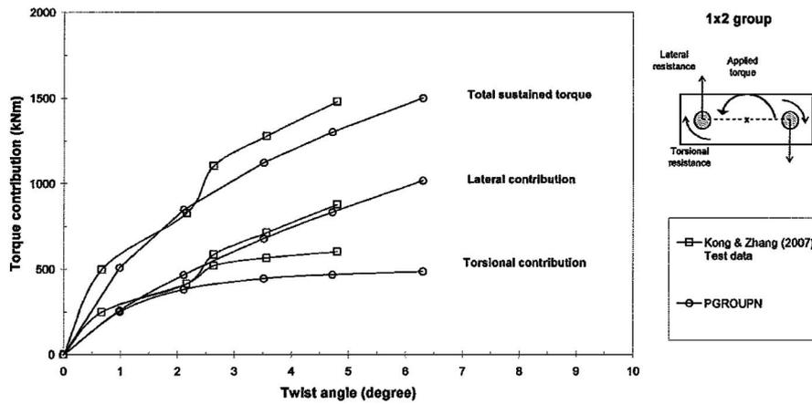
Fig. 17. Components of sustained torque in 1 × 2 pile group in dense sand
