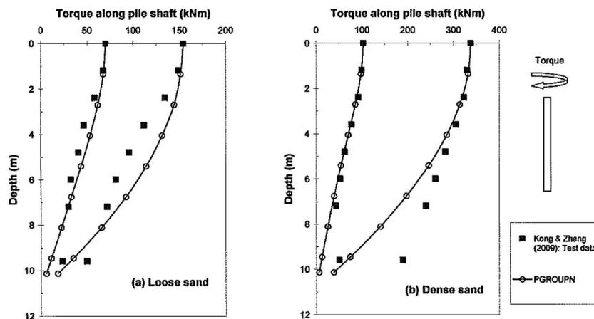
Fig. 14. Torque distribution along depth for single pile
