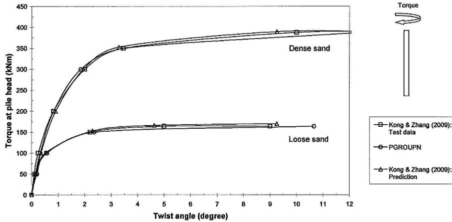
Fig. 13. Torque-twist angle curves for single pile
