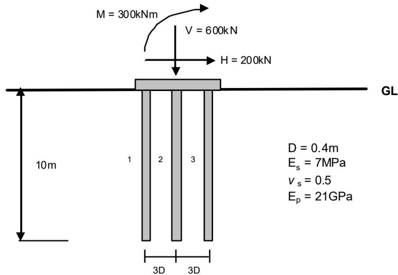
Figure 2. Group of 3 piles under general loading conditions
