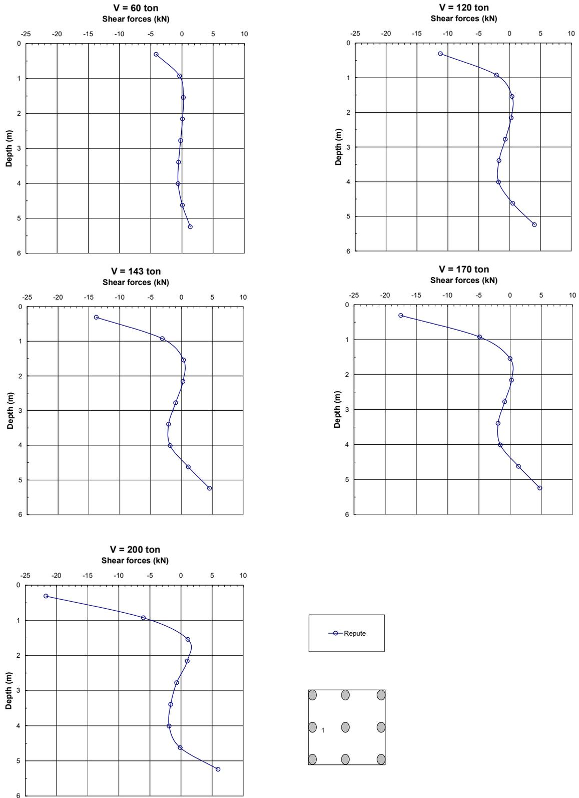
Figure 5: Shear forces on Pile No. 1 of 9-pile group
